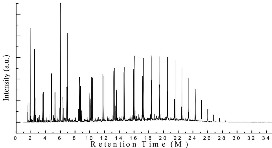
**Figure 2:** GC/MS chromatogram of mixed waste plastics and 5% ferric carbonate mixture to fuel
