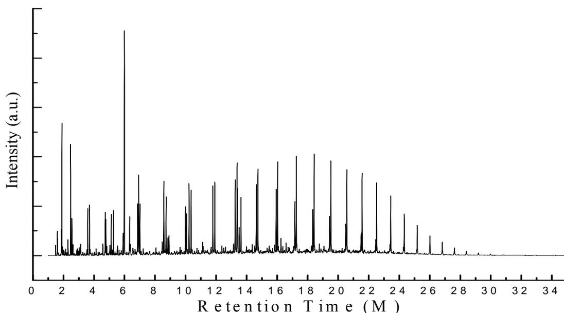
**Figure 3:** GC/MS chromatogram of mixed waste plastics and 10% ferric carbonate mixture to fuel
