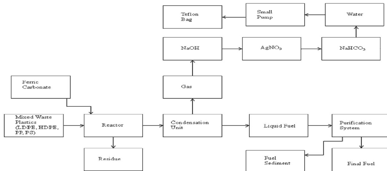
**Figure 1:** Mixed waste plastics and ferric carbonate catalyst mixture to fuel production process
