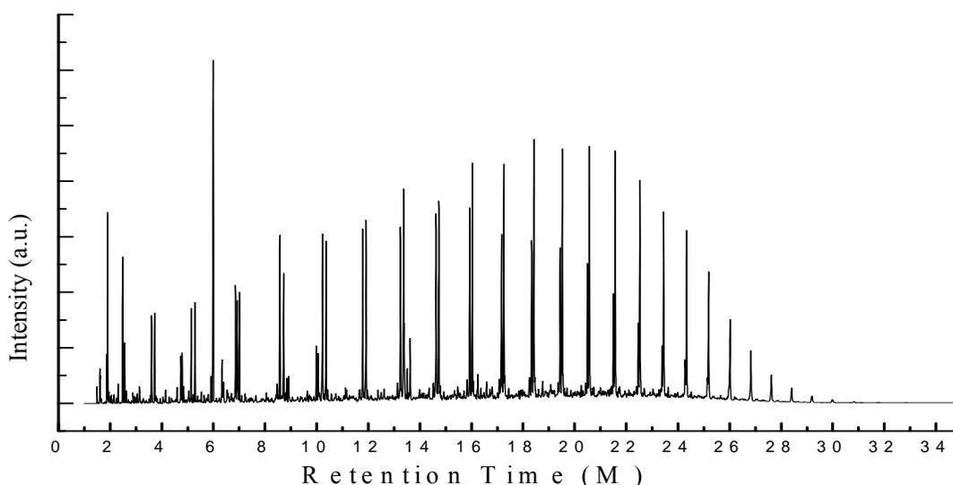
**Figure 4:** GC/MS chromatogram of mixed waste plastics and 20% ferric carbonate mixture to fuel
