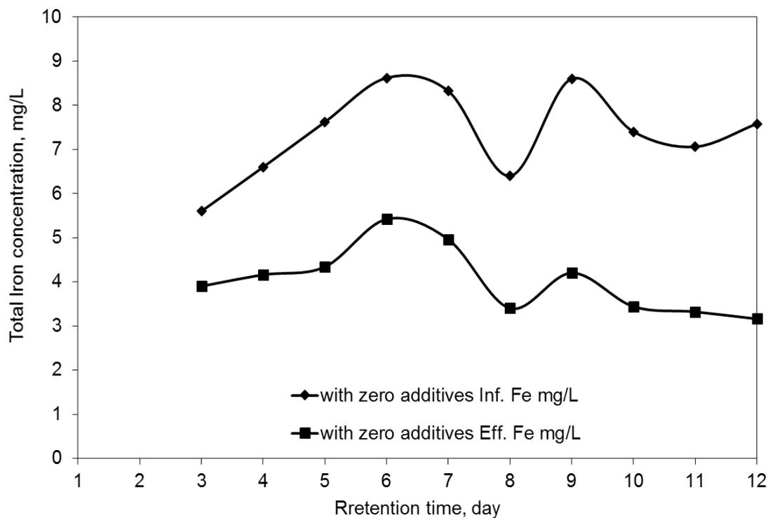
**Fig. (7):** Influent and Effluent Fe during the first group (zero additives)
