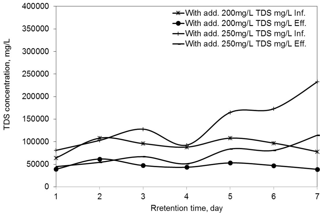
Fig. (4): Influent and Effluent TDS during the second group (with 200 and 250mg/L Alum. salts addition)
