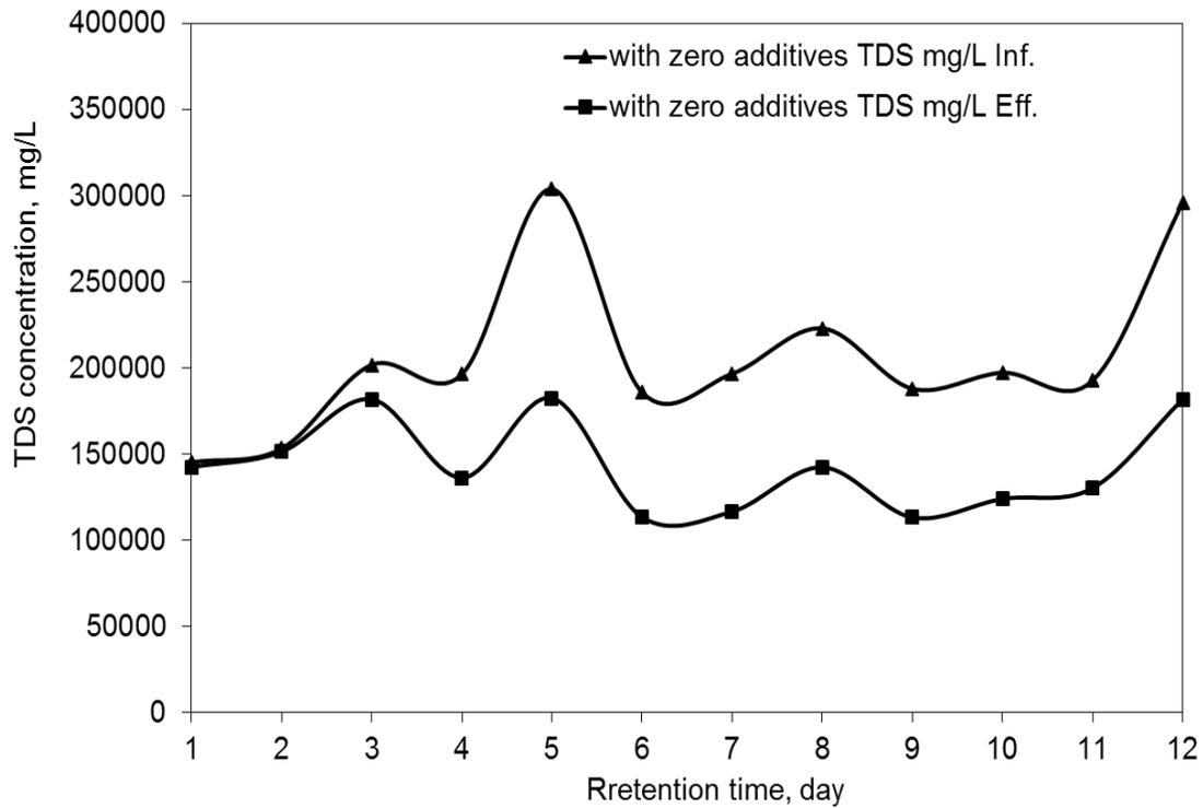
Fig. (2): Influent and Effluent TDS during the first group (zero additives)
