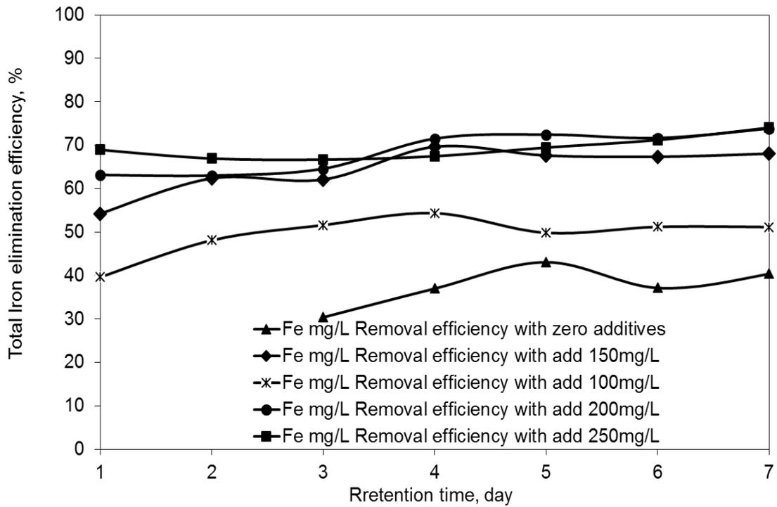
**Fig. (10):** Fe Elimination values during Alum. Salts addition for dosages from 0 to 250mg/L
