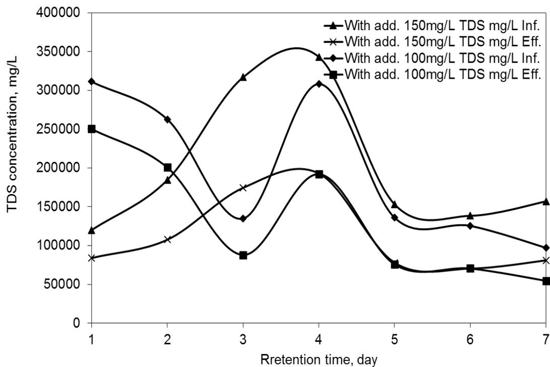
Fig. (3): Influent and Effluent TDS during the second group (with 100 and 150mg/L Alum. salts addition)
