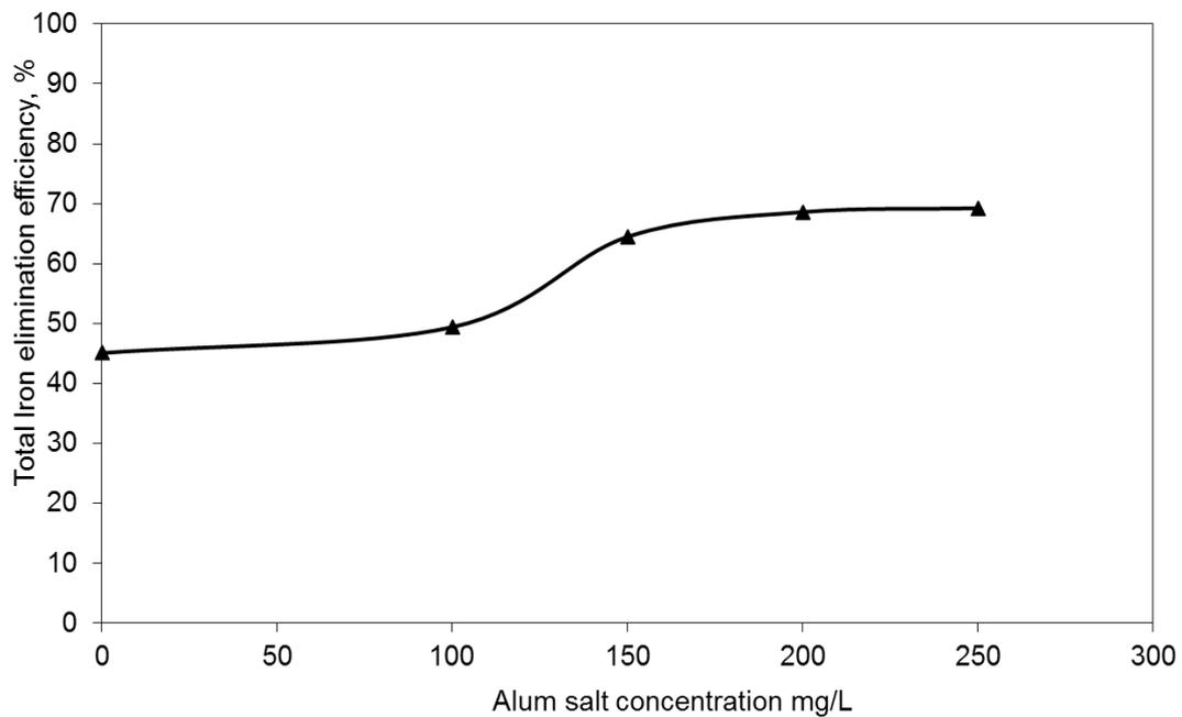
**Fig.(11):** Average Fe Elimination Efficiency values during Alum. Salts addition for dosages from 0 to 250mg/L
