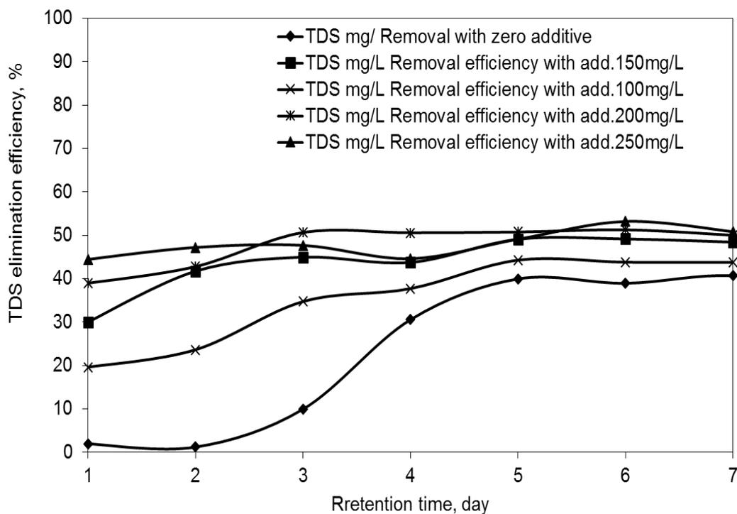
Fig. (5): TDS Elimination values during Alum. Salts addition for dosages from 0 to 250mg/L
