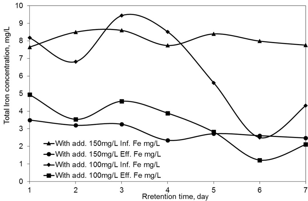
Fig. (8): Influent and Effluent Fe during the second group (with 100 and 150mg/L Alum. salts addition)
