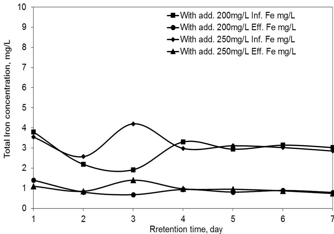
Fig. (9): Influent and Effluent Fe during the second group (with 200 and 250mg/L Alum. salts addition)
