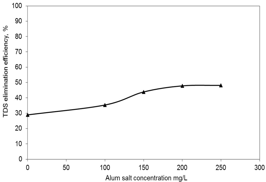
**Fig.(6):** Average TDS Elimination Efficiency values during Alum. Salts addition for dosages from 0 to 250mg/L
