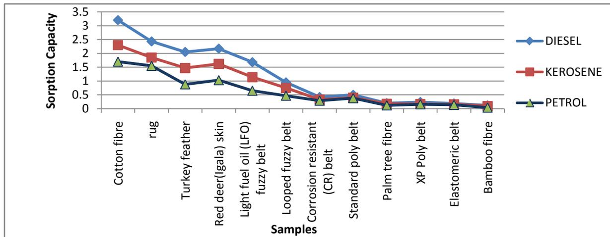
**Figure 2:** Sorption Capacities of All Samples in the Three Sample Oils
