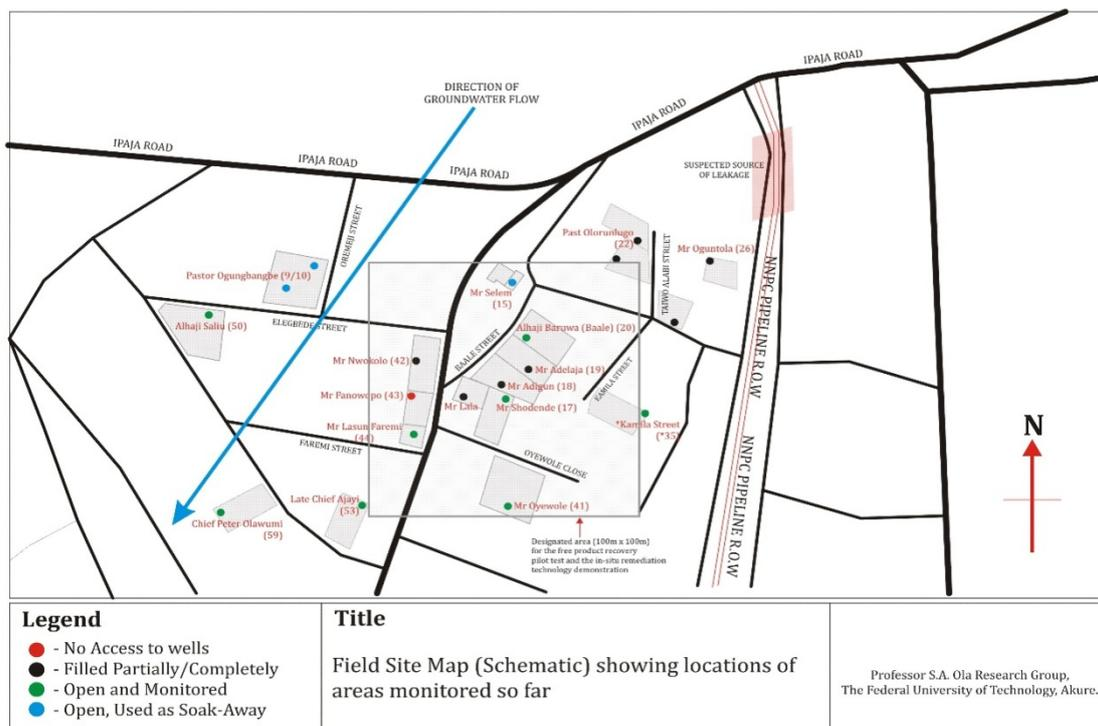
Fig 1b: Field Schematic showing Locations of Wells Monitored and Direction of Groundwater Flow (2014)
