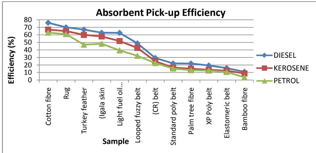
**Figure 4:** Comparisons of Pick-up Efficiencies of All Samples (Synthetic and Local) in a Mixture of Water and Fuel
