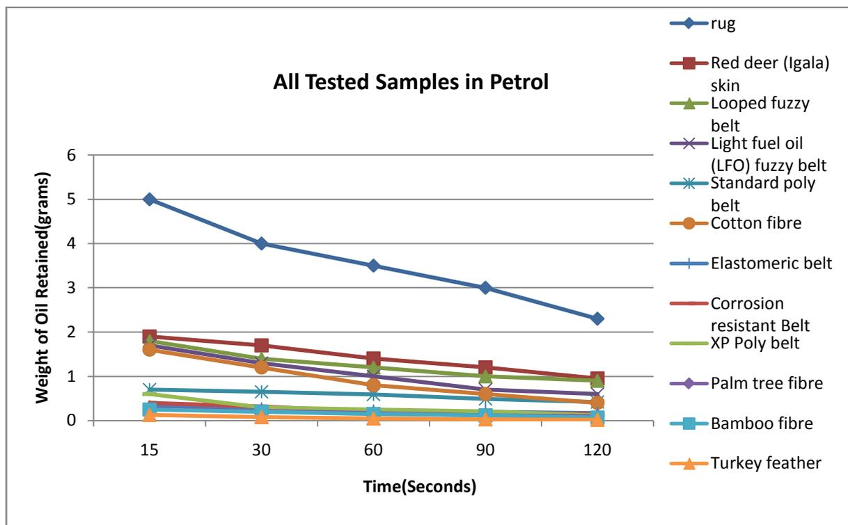
**Figure 3:** Variation of Weight of Petrol Fuel Retained with Time on All Tested Samples
