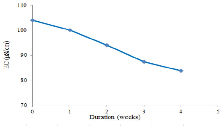
**Figure 2:** Effect of vermiremediation on wastewater contaminated with diesel engine oil's EC
