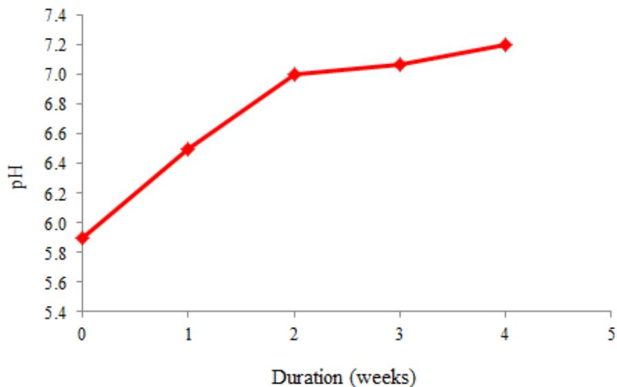
**Figure 1:** Effect of vermiremediation on wastewater contaminated with diesel engine oil's pH
