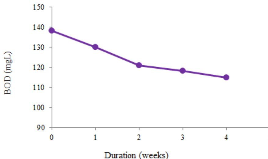
**Figure 4:** Effect of vermiremediation on wastewater contaminated with diesel engine oil's BOD
