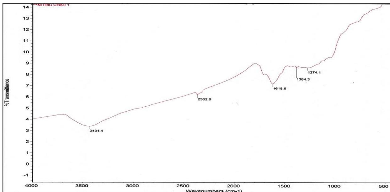
**Figure 3:** FTIR spectrum of charcoal modified with nitric acid
