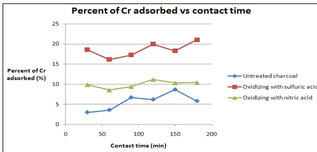
Figure 5: Graph of contact time vs percent removal
