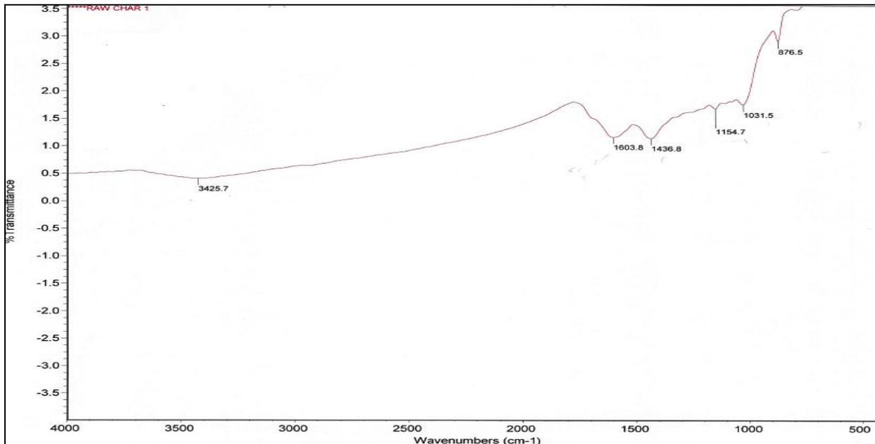
**Figure 1:** FTIR spectrum of untreated charcoal
