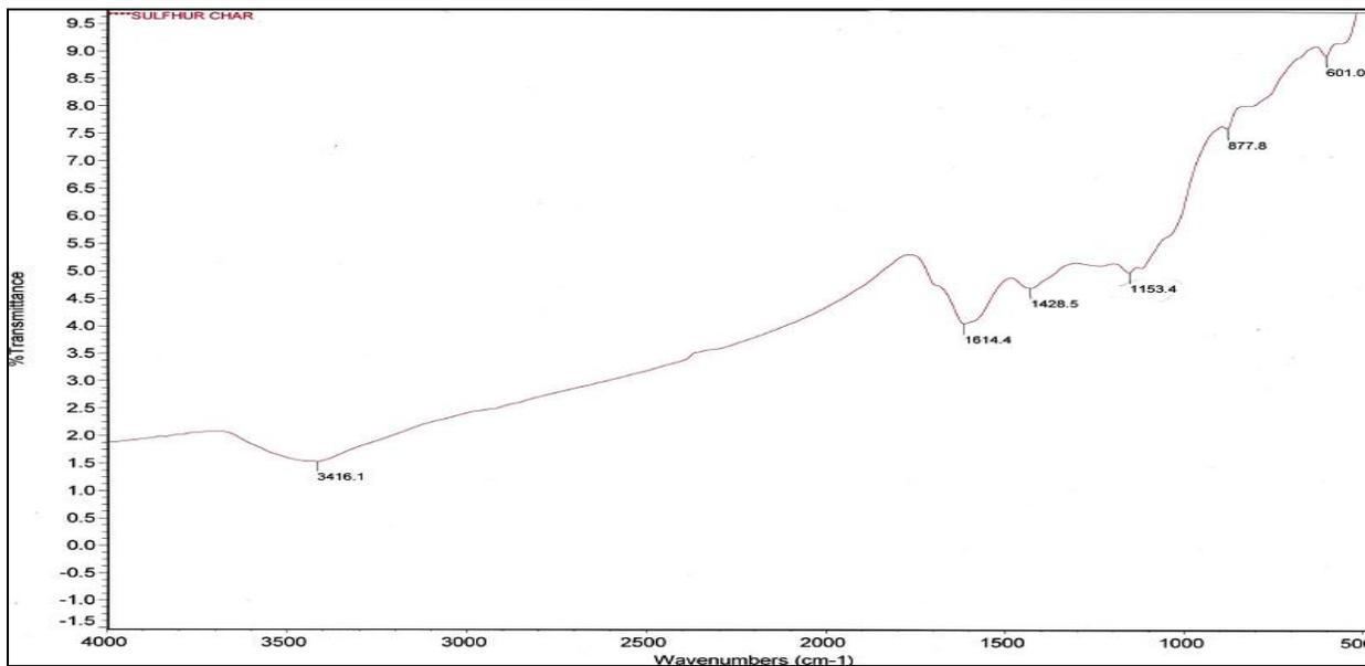
**Figure 2:** FTIR spectrum of charcoal modified with sulfuric acid
